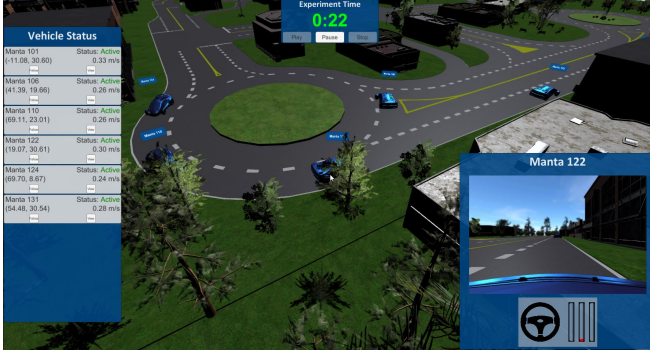
Fig. 3. The digital simulation UI during one run of the experiment. The vehicle UI nodes are on the left, the experiment controls on top, and the preview panel on the right.
